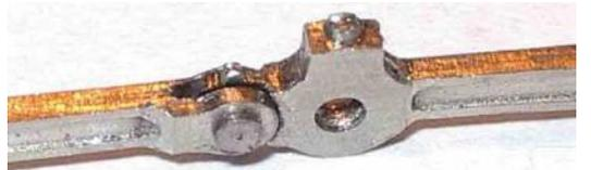
9. To stop solder flooding the joint apply a little oil to the surfaces not to be soldered - this will prevent the solder running into the joint. Keep the rear of the rod clean. Solder can then be quickly applied with a very hot iron to the back of the rod to fix the wire in place. Clean off excess solder leaving enough to keep a strong joint. See photo above of completed rods.
