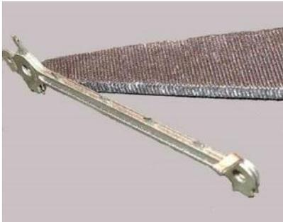
3. Open the crankpin holes using a 1.5 mm drill. When complete drill a hole using the same size drill perpendicular in a scrap piece of wood. Leave the drill in the hole in the wood. Tin the mating surfaces of a pair of coupling rods and place over the drill. This holds one end of the rods accurately ready for soldering. **It is critical to align the two halves exactly** in order to make one rod so take some time tweaking. See photo.
