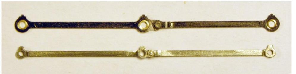
12. Fit the rods to the wheels and test run. A comparison between the Bachmann rods (lower) and the replacements is shown in the photo.
