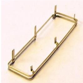
For the open cab version, take the chosen coal rails ([2] for the dropped section version or [1] for the gapped version) and push through the rivets using the half-etched holes. Position the coal rails along the back of the jig and curve the corners around the wire, one corner at a time. Check that the corner radius is tight and at 90 degrees. We used a 1.0 mm drill to help with this. For the continuous rails, attach the two ends to each other.
