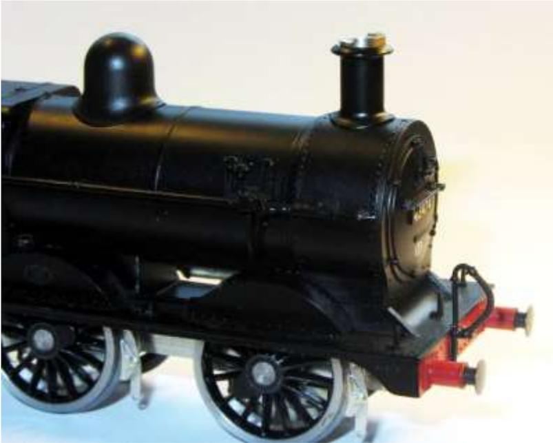
8.8.1 Remove the plastic top to the chimney by filing away the raised rim, and continuing until the flat area is the same diameter as the capuchon.
