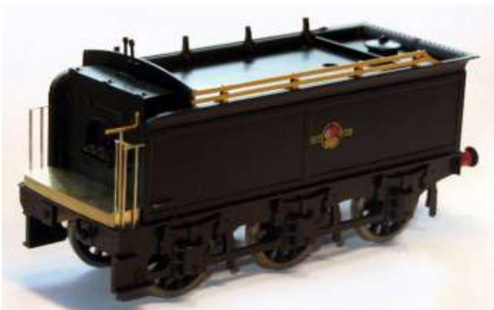
9.3.19 If fitting to the Bachmann tender frames, extend the slots in the Bachmann tender frames that receive the hooks at the front of the tender top towards the rear of the tender so that the tender top can be inserted without tilting so far. This enables the top to be taken on and off without damaging the handrails.
