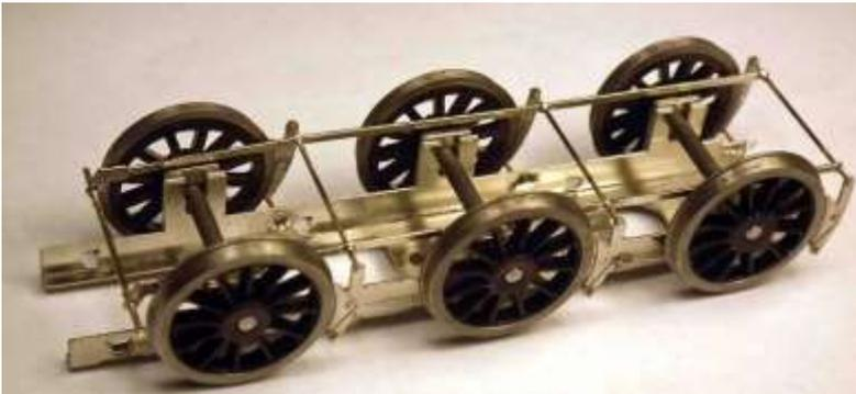
9.1.4 Remove the blocks & hanger assemblies from the etch carriers and solder to each wire cross shaft with the hanger 'short length up' in line with the wheels. Make sure that the brake blocks do not touch the wheels. Remember the wheels move up and down in the EasiChas.
