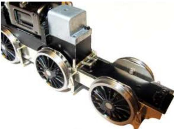
8.2.12 Remove the weightshaft assembly, trim the wire at the lever end, then attach the weightshaft assembly to the top of the Bachmann chassis block using cyanoacrylate glue or epoxy resin ensuring it fits between the dummy frames on the Bachmann footplate when the body is replaced (see photo)
