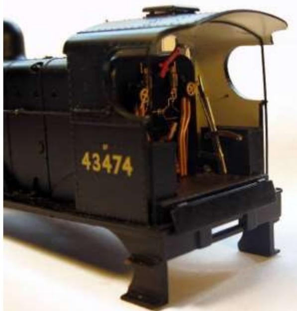
8.5.4 Remove right hand box from the cab. This is best done after removing the boiler and cab from the footplate (see 8.2.1) and remove the moulded oil boxes and pipes. Reduce the width by 2 mm by cutting with a piercing saw and finishing to size with files and emery paper. Reduce the size of the left hand box, but do not remove the moulded oil box and pipework
