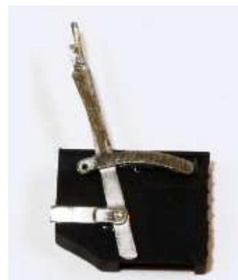
8.5.5 Attach the reversing lever to the right hand side box with the end of the quadrant 1mm in from the rear edge of the side box using cyanoacrylate glue or epoxy resin. (see photo). Trim reach rod to length.
