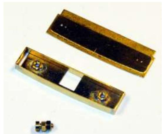
9.3.4 Curve the front footplate support front [D34] to match the curve on the underside of the front footplate [D34]. Ensure that it fits between the side pieces of the front footplate support [D33] before soldering it in place. (see photo)
