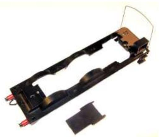
8.2.1 To fit the dummy weightshaft the footplate on the Bachmann body between the frames and between the leading and centre axle splashers needs to be removed. This is best done with a piercing saw after first splitting the body and footplate by undoing the screw under the smokebox and the cab floor, the cab handrails are glued into the cab front so carefully break the glue joint. (see photo)
