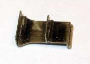
8.1.1 Bend the first bend from the top of the footstep backplate [D1] back on itself. Note bend line is on the outside. Bend the footstep back at 90 degrees at the second bend line. Ensure that the footstep fits up behind the footplate valance in the correct position.
