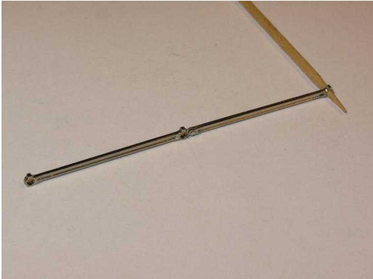
9. Open up the crankpin holes in order that the rod will either rotate on the crankpin screw (if using Bachmann wheels) or on the crankpin bushes (if using Alan Gibson or Ultrascale wheels). This can be done with a reamer, broach or a fine Swiss file.
