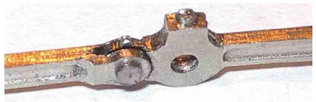
To stop solder flooding the joint apply a little oil to the surfaces not to be soldered - this will prevent the solder running into the joint. Keep the rear of the rod clean. Solder can then be quickly applied with a very hot iron to the back of the rod to fix the wire in place. Clean off excess solder leaving enough to keep a strong joint. See photo above of completed rods.
