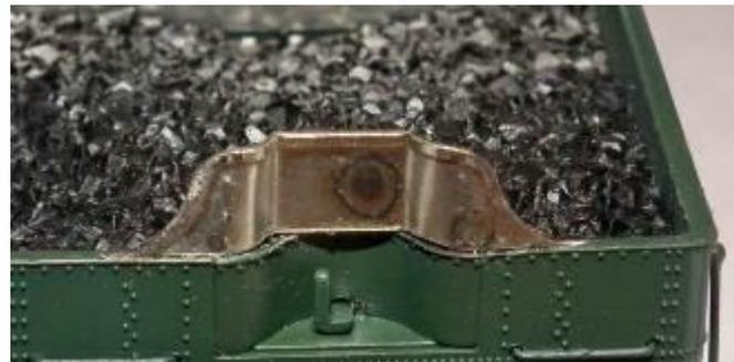
12.4 Attach the fender centre bracket [D26] to the middle of the straight section so that the rivets on the fender align with those on the bracket. Repeat for the two fender side brackets [D27].
