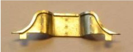
12.3 Curve the outer ends of the fender again to match the drawing Diagram 4. Note that the profile does not simply follow the line of the lamp iron recess - see prototype photo.
