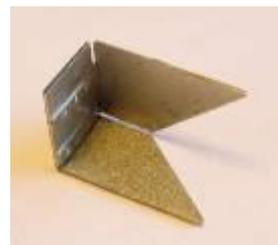
10.4 Fold the side section (the one with the two slots) up at right angles, then fold the other section up at right angles. Repeat for the other bracket.
