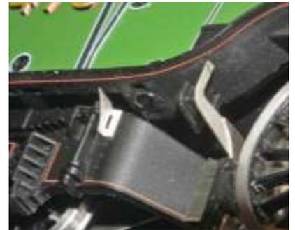
6.4 Fold the smaller bracket [D15 and D16] to 90 degrees along the slots with the bolt detail on the inside of the bend and fit to the Cartazzi truck frame immediately in front of the moulded spring hanger in-line with the rivets and with the riveted flange towards the front of the loco (see photo above). Fix using cyanoacrylate or preferably epoxy resin (the plastic is difficult to fix to and fixing is helped by scoring the plastic).
