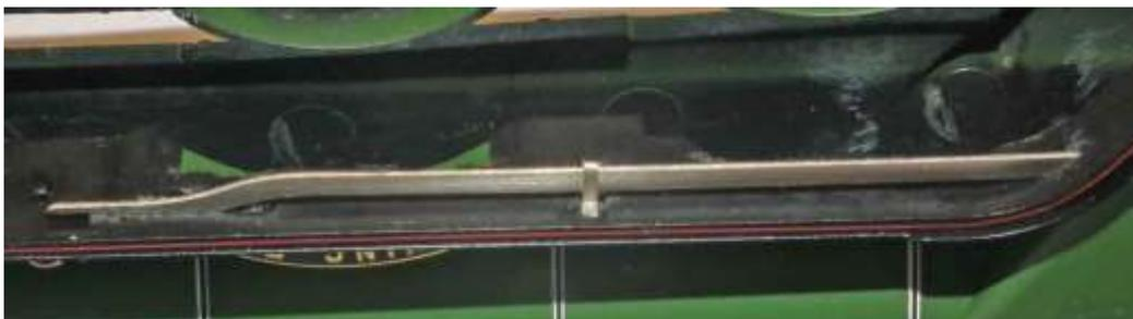
reach rod with no joint plate fitted to the Hornby body.
