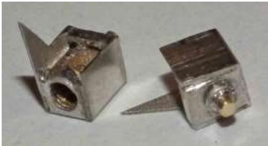
4.8 Cut two short lengths of 1.0 mm diameter wire. Insert the wire through the buffer washer [D8] and the smaller hole in the end of the buffer spring housings ensuring that the wire does not protrude into the tube. Trim the wire to length. Solder together (see photo of the finished assemblies).
