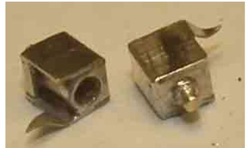
Ensure that the larger hole in the end of the buffer spring housing and tube pass over the inner end of the Hornby buffer – open up if necessary with an appropriate size drill. Do not attach to the chassis overlays at this stage.
