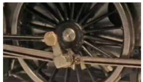
11.3 Reduce the thickness of the rivets connecting the eccentric rods to the return cranks.
