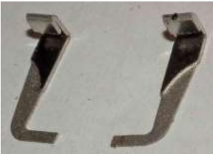
6.2 Fold up the larger bracket [D13 and D14] by first folding the small outer section back on itself with the fold line towards the outside of the bend, and then bending at 90 degrees at the second bend line with the bend line to the inside of the bend. See Photo left.
