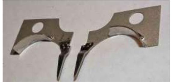
4.4 Make sure the etch cusps are removed from each side of the thin arms of the buffer spring housings [D6 and D7].
