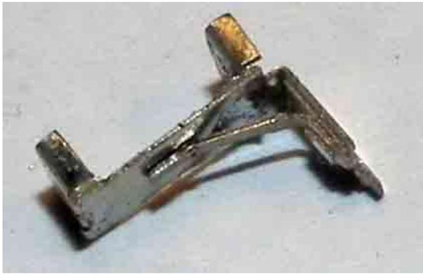
5.5 Bend the step supports as shown in photo left, making the bends at the end of the half etched section and at the small hole in the half etched section. Solder to the base of the footsteps. See photo right.
