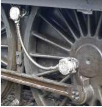
9.1 Late in their career some locos were fitted with BR speedo equipment. See photo. A casting for the speedo drive is available separately from Brassmasters if required for the period modelled. The support bracket is provided as part of the detailing kit.
