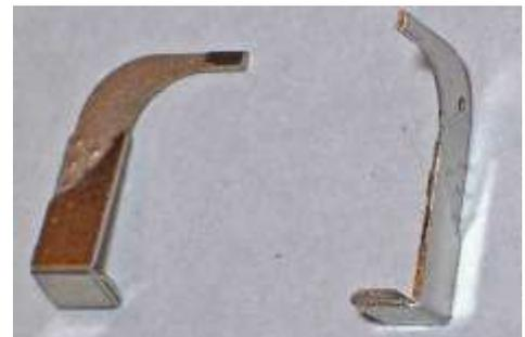
6.3 The representation of part of the bracket moulded on the front of the firebox sides of the Hornby body will need to be removed to clear the new bracket. See Photo 9, original on left, bracket filed off on right (damper lever is also removed).
