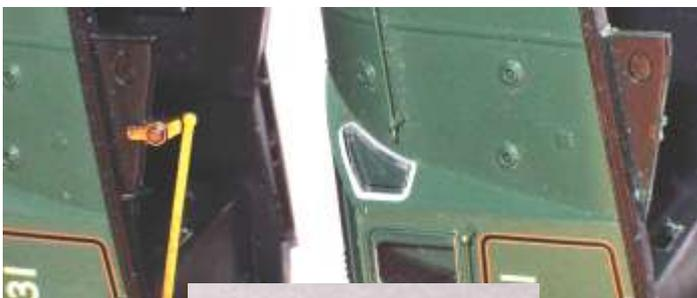
6.4 Re-attach the body. Attach the brackets to the outside of the Hornby chassis, using cyanoacrylate or epoxy resin, with the bent tab behind the wheel so that the bracket is just above and level with the rear of the plastic brake hanger and using the loco footplate as a guide. (As a check, the bracket with the small hole is fitted to the right hand side of the loco). See Photo 11
