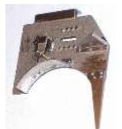
4.3 Solder the splashers into position. The angled corner should be to the outside and towards the front of the loco.
