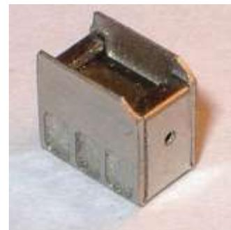
4.7 Take the triangular buffer beam brackets [D7]. Solder to the two chassis overlays above the riveted strip. (Note - Photos 1 and 2 show the test assembly where the brackets had a fold over front edge. The kit ones do not.)
