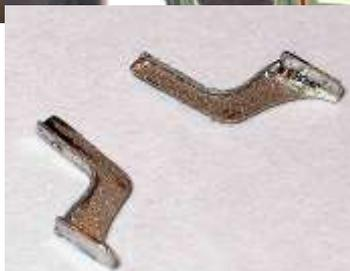
the smaller bracket [D22 and D23] to 90 degrees along the bolt detail on the inside of the bend.
