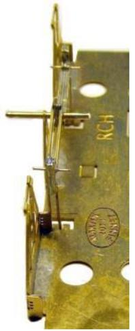
The wire between the 'V' hangers now needs to be removed. To cut off the 0.8mm wire brake shaft between the two sets of brake gear **DO NOT CUT THE WIRE WITH SNIPS** as it will distort the 'V' hangers – make the first cut with a saw. The second cut can be made with snips. The wire should be cut back to just behind the push rods.
