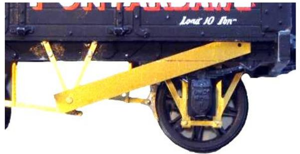
There are two common types of brake lever guide support strap fitted between the bottom of the brake lever guide and the 'W' iron. These either go to the bottom of the 'W' iron keeper plate [U16] or part way up the 'W' iron [U17]. Take the appropriate etches and fold as shown in the photos (the bends are quite severe!). When satisfied with the shape solder the straps to the bottom of the brake lever guide.
