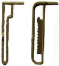
Decide which type of brake lever guide is required, pin type [U14] or ratchet type [U15]. Bend to shape as shown in the photo using the half-etched marks. The bottom bend of the pin type should be bent first by placing in the slot in the brake lever guide jig and bending over so that both sides lay flat along the jig. This should give a nice round curve.
