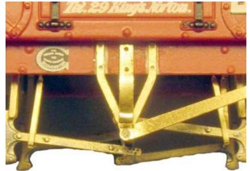
drilled out 0.4 mm. Bend as shown in the photo (we used a 5mm drill for the larger radius and round nose pliers for the smaller radius). The large bend starts 3.25mm from the top.
