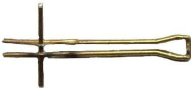
Carefully bend the brake hangers, as shown in the photo, at the half-etched marks on the inside and outside of the etch. It is essential that when a piece of 0.3mm brass wire is passed through the two holes in the middle of brake block it is parallel to the top, so don't be afraid to persevere until it is.
