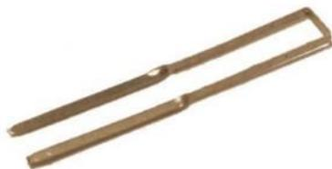
The legs on the safety loop need to be 10.5 mm long. Cut the legs to the appropriate length. Solder the safety loops into the slots in the subframe base, towards the outer end for P4 and EM, at the inner end for 00.
