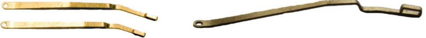
Cut the brake lever guide jig [U13] from the side of the etch (see photo below). Open out the large hole to clear the brake shaft and the small hole 0.5mm.
