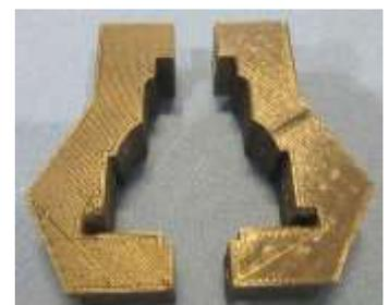
This part can be clamped around the Hornby body and holds the drill at the correct angle and in the correct place for drilling the holes for the knobs.
