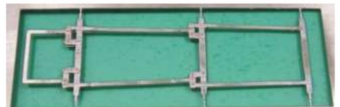
16.9. Once the brake pull rods are complete, remove from the fret and slightly round the corners of the ends of the tie rods so that the ends will fit into
