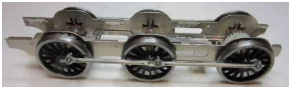
the bench without it binding. If it is binding, check the quartering and check each crankpin in turn to see which one is stuck. If required, then slightly open up the crankpin hole in that rod. Do this carefully and a little at a time, you can easily remove material -putting it back is a lot harder.
