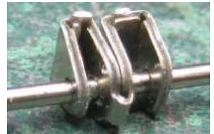
**Note that these hangers are handed**, the more angled face is orientated towards the outside of the chassis.
