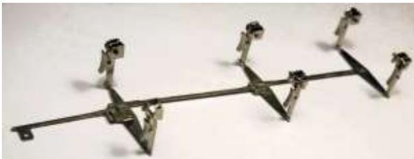
through the frame. This will allow the whole unit to be sprung off the chassis so that the wheels can be removed. Test fit the chassis on the footplate. The brake hangers will be hard up against the footplate, file and adjust as necessary.
