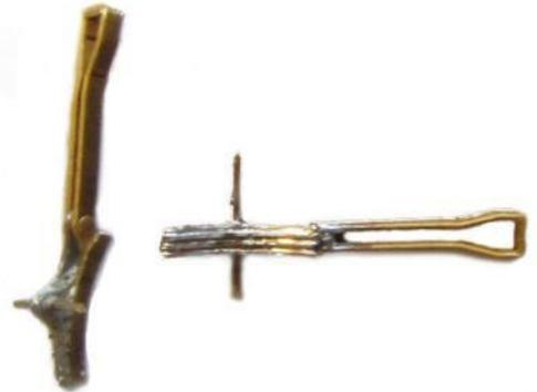
Solder the brake hanger assemblies in place in the 'E' shaped openings in the subframe floor, the outer slots for P4 and EM, the inner ones for 00. The floor will now need to be recessed to clear the brake hangers where they protrude above the subframe floor. This is done using a large drill rotated in the fingers.
