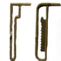
Cut the brake lever guide jig [U16] from the side of the etch. The point at the end may need to be removed for some wagons. Open out the large hole to clear the brake shaft and the small hole 0.5mm. place the jig over the brake shaft, align the etched line on the jig with the bottom of the solebar and spot through the 0.5mm hole with a 0.5mm drill. Drill through the sole bar 0.5mm.
