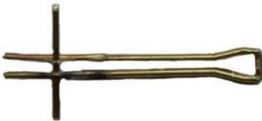
Mount a brake block centre [U4] between the brake blocks with a piece of 0.3 wire protruding from both sides, align the brake block centre with the brake blocks and solder together. Leave the wire protruding from each side. Repeat for the other brake block hanger assemblies.
