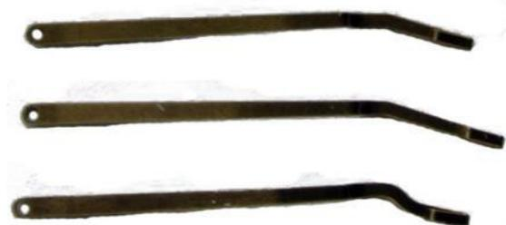
There are three types of brake lever on the etch, short standard [U11], long standard [U12] and cranked [U13]. Take the appropriate lever(s) and bend to shape as shown in the diagram, using the half etch lines and dots as a guide.
