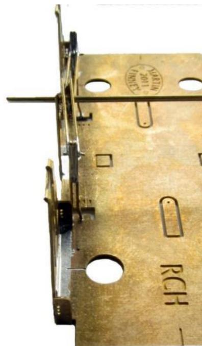
For single sided brakes, snip off the 0.8mm wire just behind the pull rods. **FOR DOUBLE SIDED BRAKES DO NOT CUT THE WIRE WITH SNIPS** as it will distort the 'V' hangers – make the first cut with a saw. The second cut can be made with snips. Again, the wire should be cut back to just behind the push rods.
