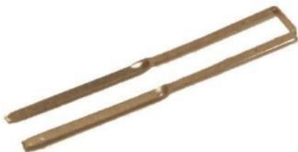
For different length safety loops take one or two safety short loops [U8] and bend at right angles at the two half etched marks in the centre of the loop. Hold one leg of the safety loop below the half-etched mark on the leg in a pair of pliers and twist the leg above the pliers through 90 degrees. Repeat for the other leg. Repeat for the longer length safety loop(s) [U9].
