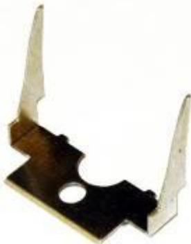
10.22 Fold up the replacement guard irons [T3] by firstly bending the section with a 'U' shaped cut-out through 180 degrees back on itself **with the half etch bend line to the outside**. Then bend up the two guard irons at right angles and then bend to shape. Finally file a small amount off the top of the step where the guard irons fit around the bottom of the buffer beam ( there is a small mark on the etch indicating where to file but not how much) (see photo 10.22)
