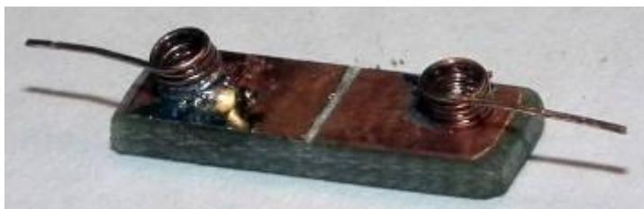
phosphor bronze wire (not supplied but available from Eileens Emporium), wind a 'spring' shape with extended end. I clamp a fine screw driver in the vice and holding the wire one end in the fingers and the other in a pair of round nose pliers, form the spring round the screw driver shaft. Note one pickup is wound clockwise, one anti-clockwise. Solder to the copperclad (gapping it first!) as the photo above.
