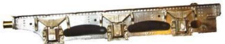
10.14 Solder the rivet detail fronts [F15 and F16] in place on each side of the frame
