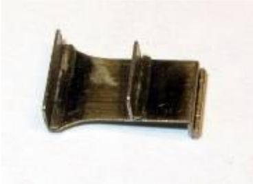
8.1.1 Bend the first bend from the top of the footstep backplate [D1] back on itself. Note bend line is on the outside. Bend the footstep back at 90 degrees at the second bend line. Ensure that the footstep fits up behind the footplate valance in the correct position.
