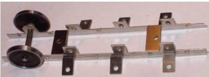
6.11 Fold up the replacement guard irons [T3] by firstly bending the section with a 'U' shaped cut out through 180 degrees back on itself **with the half etch bend line to the outside**. Then bend up the two guard irons at right angles and then bend to shape. Finally file off the two small tabs between the guard irons. (see photo)
