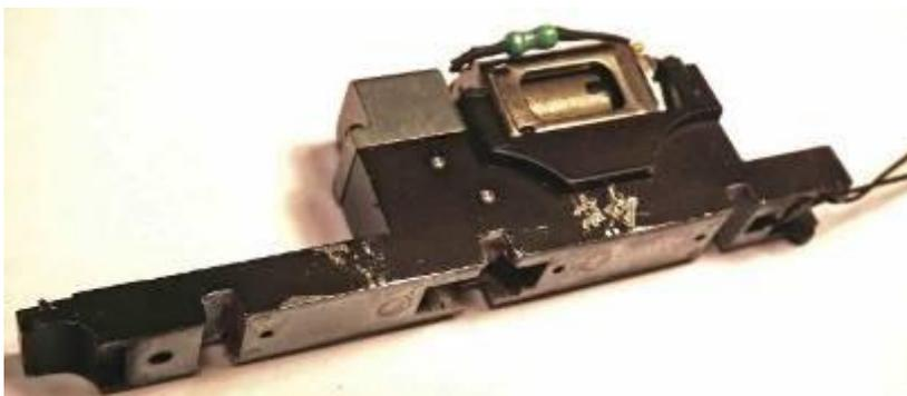
3.7 Remove the wheel sets from the chassis, unscrew the machine screws from the wheels and remove the coupling rods. Put the screws back into the wheels for safekeeping. The chassis should now look like the photo. De-grease the chassis sides.
