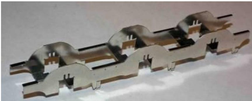
5.2 Remove the loco mainframes [L1] and clean up the residual tabs with a small file.
