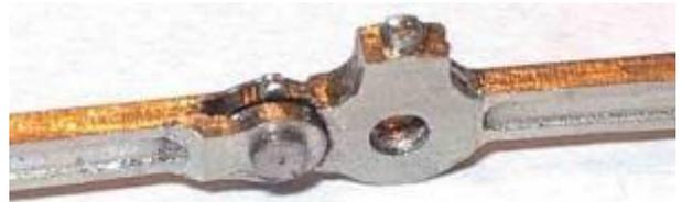
To stop solder flooding the joint apply a little oil to the surfaces not to be soldered - this will prevent the solder running into the joint. Keep the rear of the rod clean. Solder can then be quickly applied with a very hot iron to the back of the rod to fix the wire in place. Clean off excess solder leaving enough to keep a strong joint. See photo above of completed rods.
