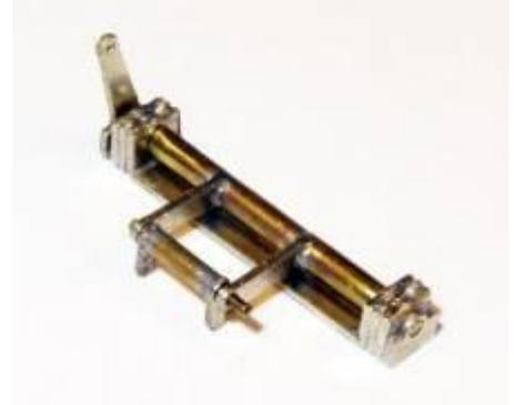
If the weightshaft is assembled in mid gear the small end of the weightshaft levers should be held off the flat surface by the lifting links. Solder up the weightshaft assembly in this position. (see photo right)
