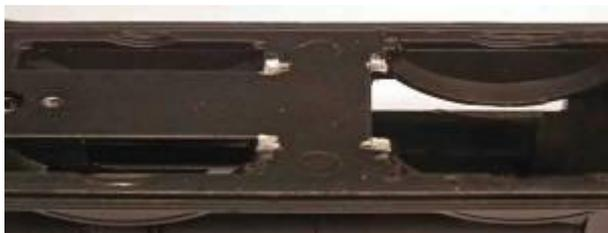
5.19 In order for the chassis to sit properly under the footplate file off the 4 'pips' under the footplate between the splashers. See photo below – they are the 'shiny' bits.
