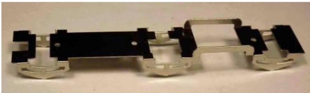
5.6 Test fit the keeper plate and the chassis to the Bachmann chassis.
