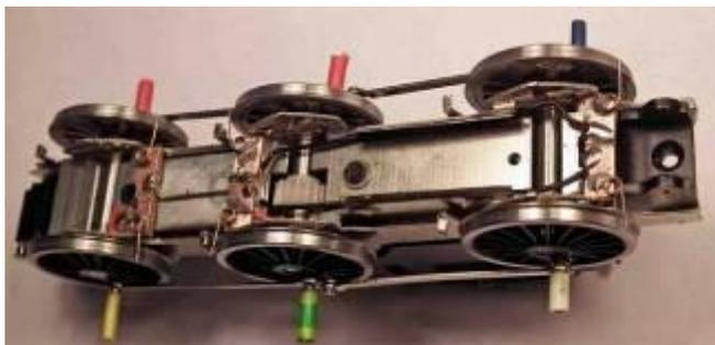
5.21 Glue these to the chassis keeper plate in the position shown in the photo below so they gently press on the wheel flanges. Test the polarity and direction of travel with another loco and connect together and to the motor with wire. Test Run. When happy remove the temporary crank pins, shorten the bushes and fit the crankpin bushes (note, if you are going to fit new coupling rods as per section 7.1 do **NOT** shorten the bushes).
