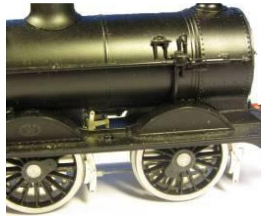
8.2.11 Attach the reach rod lever to the inside of the plastic frame using cyanoacrylate glue or epoxy resin
