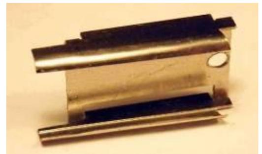
5.8 Curve up the half etched sides of the ash pan [L3] with the half etch to the inside. Fold up the ashpan into an inverted U with the side curving in towards the middle. See photo.
