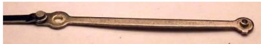
Fit the rods and temporarily secure with a piece of electrical wire sleeve (does not come unscrewed unlike a proper 14BA nut!). The rod with the joint (as Photo) is the trailing rod on both sides. Check that all the wheels now turn without binding when power is applied to the motor and are quartered correctly. Be careful as you tighten the retaining screws
