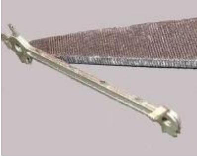
7.1.3 Open the crankpin holes using a 1.5 mm drill. When complete drill a hole using the same size drill perpendicular in a scrap piece of wood. Leave the drill in the hole in the wood. Tin the mating surfaces of a pair of coupling rods and place over the drill. This holds one end of the rods accurately ready for soldering. It is critical to align the two halves exactly in order to make one rod so take some time tweaking. See photo.
