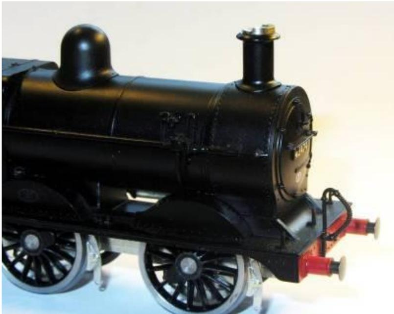
8.8.1 Remove the plastic top to the chimney by filling away the raised rim, and continuing until the flat area is the same diameter as the capuchon.
