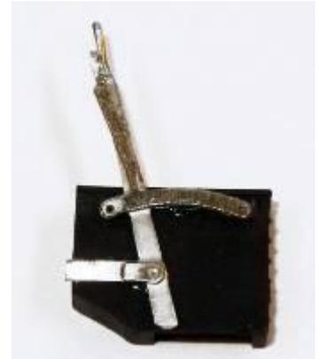
8.5.4 Remove right hand box from the cab. This is best done after removing the boiler and cab from the footplate (see 8.2.1) and remove the moulded oil boxes and pipes. Reduce the width by 2 mm by cutting with a piercing saw and finishing to size with files and emery paper. Reduce the size of the left hand box, but do not remove the moulded oil box and pipework
