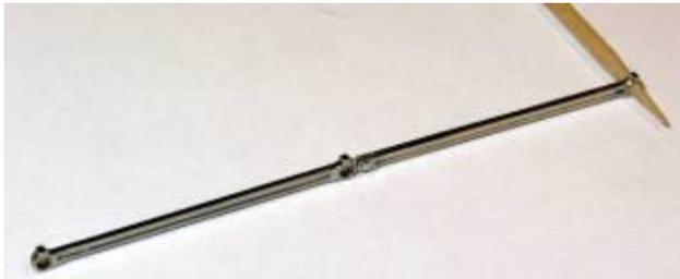
Open up the crankpin holes in order that the crankpin bushes will rotate in the rod. This can be done with a reamer, broach or a fine Swiss file.
