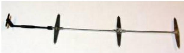
5.23 Take the brake pull rod etch [L6], identify the three overlays representing the linkage each side of the cross shafts [L7 for the front fork end, L8 for the middle shackle and L9 for the rear shackle]. Push through the rivets in the middle and back overlays [L8 and L9], then solder or glue the top and bottom overlays to the pull rod. Find the Bachmann plastic pull rod assembly and cut it immediately behind the rear cross shaft and carefully cut away a section between the two
