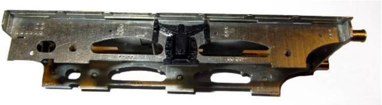
10.19 Cut the axlebox and spring hanger assemblies from the Bachmann frames using a piercing saw. Trim around the axlebox and spring. Remove the raised section on the back of the moulding and then attach to the replacement frames (see photo above)
