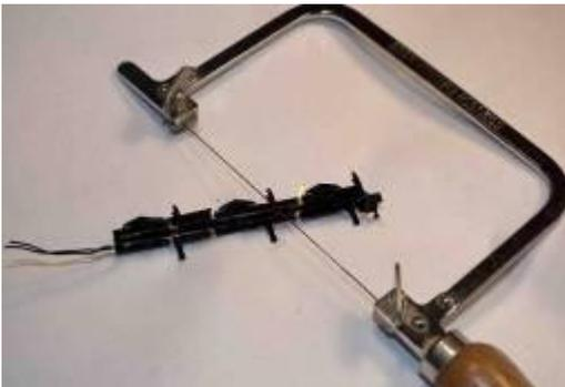
5.11 Carefully cut the brake gear off the two Bachmann keeper plates by sawing next to the main part of the centre solid section. Once the saw cut is started hold the brake block (not the bigger keeper plate) or they will ping off across the room! See photo. Keep safely for later use.
