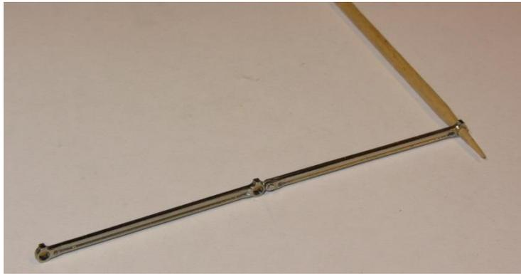
11. Open up the crankpin holes in order that the rod will either rotate on the crankpin screw (if using Bachmann or Markits wheels) or on the crankpin bushes (if using Alan Gibson or Ultrascale wheels). This can be done with a reamer, broach or a fine Swiss file.
