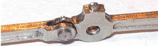
To stop solder flooding the joint apply a little oil to the surfaces not to be soldered - this will prevent the solder running into the joint. Keep the rear of the rod clean. Solder can then be quickly applied with a very hot iron to the back of the rod to fix the rivet in place. Clean off excess solder leaving enough to keep a strong joint. See photo above of completed rods.
