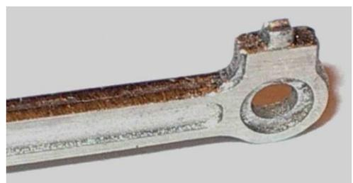
crankpin bushes (if using Alan Gibson or Ultrascale wheels). This can be done with a reamer, broach or a fine Swiss file
