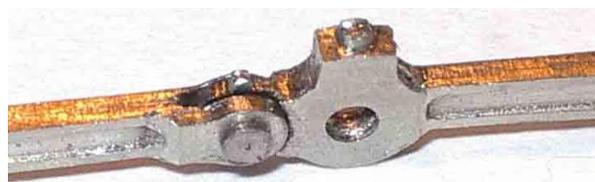
13 To stop solder flooding the joint apply a little oil to the surfaces not to be soldered - this will prevent the solder running into the joint. Keep the rear of the rod clean. Solder can then be quickly applied with a very hot iron to the back of the rod to fix the rivet in place. Clean off excess solder leaving enough to keep a strong joint. See photo of completed rods.
