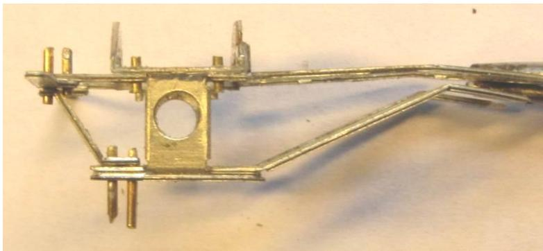
20 If fitting the ATC beams [P4], attach them to the front and back of the pony truck using 0.45mm wire.
