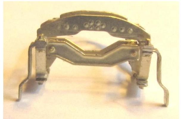
29 Curve the upper strengthening ribs [P7] to fit in the slots in the upper arms and solder into position.
