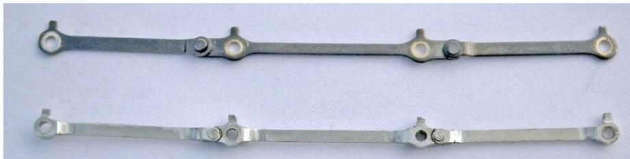
15 Open up the crankpin holes in order that the crankpin bushes will rotate freely in the rods. This can be done with a reamer, broach or a fine Swiss file.
