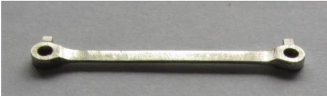
12 Open up the crankpin holes in order that the crankpin bushes will rotate in the rod. This can be done with a reamer, broach or a fine Swiss file.
