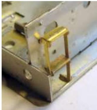
8.8.11 Attach the steps to the frames using cyanoacrylate glue or epoxy resin (see photos of the steps fitted to the similar replacement frames)..
