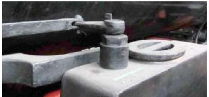
closer to the sandboxes than the left – be aware of this when you are making these mechanisms and try a 'dry run' of fitting the boiler **before securing these mechanisms**. Also, it will be necessary to carve the back of the bracket on the splasher until it is slightly thinner.
