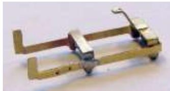
8.8.8 Bend over the tops of the supports either side level with the rearward facing tab and towards the front of the locomotive.
