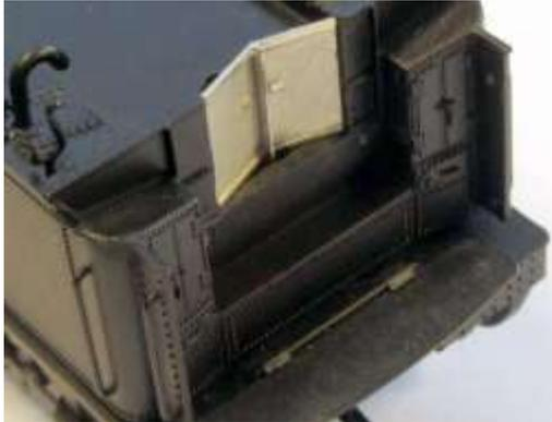
8.3.5 Make a series of holes with a drill in the coal space floor just behind the front wall between the saw cuts. Open up between the saw cuts so that piece falls out.
