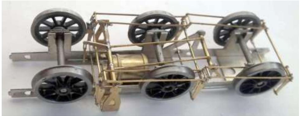
8.1.35 Remove the brake gear by springing the top of the hangers off the support wires. If you have used an active flux, remove the wheels and clean thoroughly to remove any flux.
