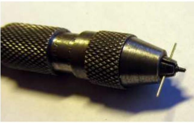
7.8.5 Carefully remove two knobs from the short end of the wire. Put one carefully away, but the other will need to be mounted in a pin chuck with the base outwards. This is best done by mounting the hand rail on a short piece of wire, putting the wire into the chuck between the jaws and then tightening the chuck on the knob.
