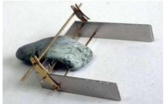
8.1.23 Push a 30-40mm piece of 0.5mm wire through the upper exposed hole in one brake hanger, then through the single hole of two brake pull rods ([D40] and [D41]) with the detail side face to face. Ensure that the rods are correctly orientated. Finally push the wire through the opposite brake hanger. Make sure that an equal amount is showing either side of the brake hangers and solder into place to the brake hanger only (not the pull rod at this stage).
