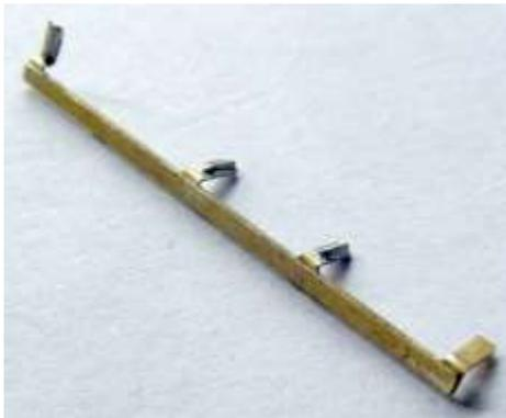
8.4.3 Turn the etch over and fill the groove in the back of the upright with solder.
