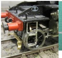
b. Bend up the ends of the step treads [D5] and then fold the sides of the loco or tender step frames around them. Solder the treads in place in place and then tidy up by filing the cusps back to thin down the thickness. Make sure there is a left hand and right hand set of steps for the tender.
