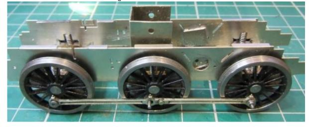
c. Once happy that the chassis rolls smoothly, the Bachmann chassis block can be reinstalled and fastened using the front and rear bolts. At this point the motor and Bachmann gear tower can be added back into the etched gear tower. If you plug the unconverted tender into the locomotive using the original Bachmann cabling you can power the chassis from the tender to test, though obviously the tender will still be OO so you might need to be creative with the track/rolling road.
