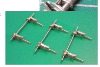
I. The brake pull linkage [L10] comes with matching half-etched linkage details [L11, L12, L13, L14] which need to be applied to the top and bottom of the main etch. It is easiest to tin the parts BEFORE removing from the main etch and to leave the pull rod
