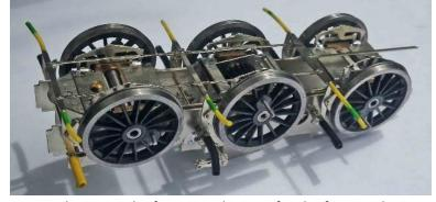
position cut the central section of the 0.8mm wire away between the frames with a saw for the first cut, leaving about 0.5mm to protrude through the frame. This will allow the whole unit to be sprung off the chassis so that the wheels can be removed.
