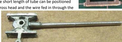
e. The pivot hole for the union link in the crossheads should be opened up to 0.6mm.
