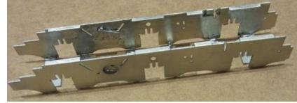
using a smooth sharp file lightly file away the cusp equally on both of the edges of the slots until the bearing slides up and down with no binding. It is very important that too much metal is not removed resulting in a sloppy fit – no side play whatsoever is the aim, just a smooth sliding fit.
