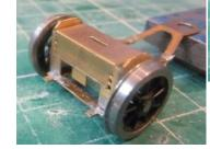
the wire through the holes in the front of the pony truck, through the slots in hornblocks and out of the holes in the rear of the pony truck. The pony truck has three pairs of holes, the lowest of which give around 3/4mm of vertical movement to the axle. Attach the pony truck wheels to the axles ensuring that you have the correct back-to-back gauge. Limit the side play using the various etched washers supplied on the etch.
