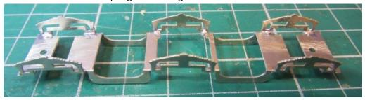
c. Test fit the keeper plate into the bottom of the main frames. You may need to file away some of the solder bead to get a good fit. Note that the keeper plate is not symmetrical, ensure that you aren't trying to force it in the wrong way around.
