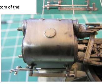
b. Before soldering to the frames, it is a good idea to fold up and test fit the cylinder connector [L41] to ensure this will fit as intended.
