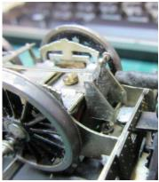
should you need to remove the brake pull rods and wheels. The brake hangers will be hard up against the footplate, file and adjust as necessary.
