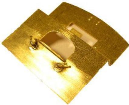
10.24 Bend the ends of the 2 handles [FD20] as seen in the photos and solder to the wire. The handles should be just under 2 mm from the tender front (see photo).
