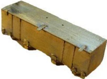
10.20 Using 0.33 mm wire bend up the handrail on the top of the toolbox and solder in place
