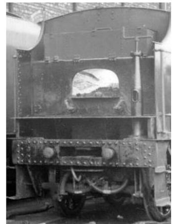
10.25 Push through the rivets in the top half of the new front for the fire iron bracket and, if being fitted, the rivets for the coal rails.
