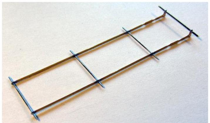
9.6 Refit to the brake hangers and check all is ok. Make sure that the brake hangers are as far apart as possible then trim the cross wires.
