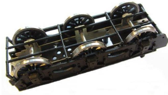
8.6 Refit the plastic brake hanger assembly to the plastic underframe using cyanoacrylate glue or epoxy resin.
