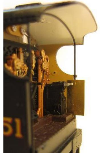
12.2 There are two lengths of tender cab doors provided. The scale size doors [FD23 and FD24] can be used when your layout curves are very large. However, for most layouts the wide cab doors [FD25 and FD26] are better.
