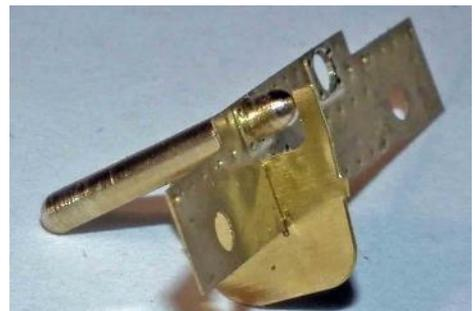
6.9 Replace the Bachmann buffers or fit replacement buffers, undoubtedly you will have damaged the Bachmann red paint so it is probably best to remove this from all the buffer body before re-fitting.
