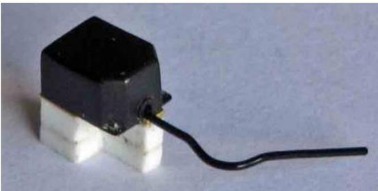
5.6 File the sides of the leading two Bachmann sandboxes so that the back edge is the same width as the front edge. Thin the boxes by rubbing the back in a circular manner on emery paper until the box is about 3.3 mm thick (if you have rubbed off the fixing lugs at the bottom you
