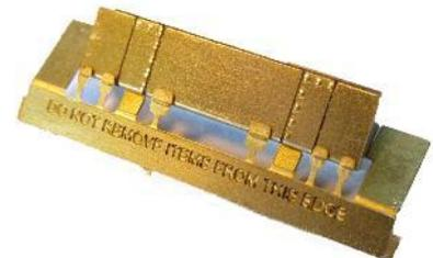
the six hinges first carefully solder all six in place.
