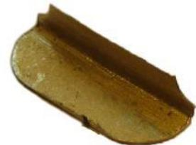
10.22 File off the nibs so that the coal plate fits through the coal hole and solder in place from the rear.
