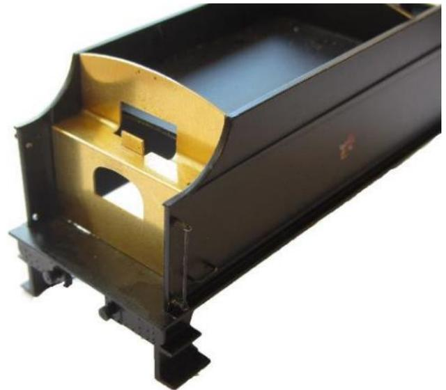
10.10 Push through the rivets in the toolbox [FD13] and the tool box top [FD14]. Fold up the tool box [FD13] into a U shape making sure the bends are 90 degrees.
