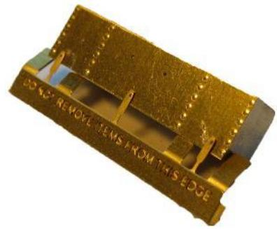
10.18 Cut the tabs to the three hasp and staples and clean up the cut edges.
