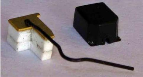
5.2 Join a piece of 4 mm x 2 mm plastic strip to a piece of 4 mm x 1 mm and a piece of 4 mm x 0.25 mm, all 7 mm long, using solvent, to form a spacer block.
